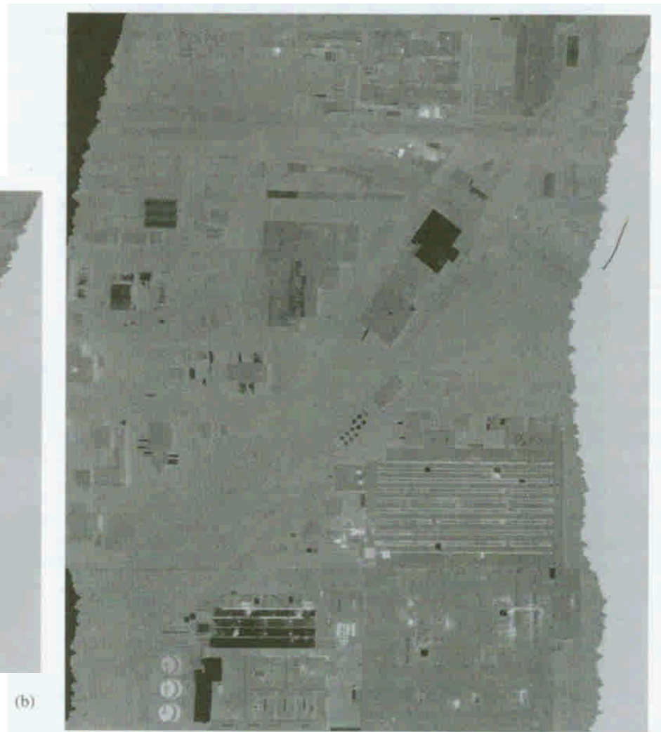
Figure 5.19 Thermal infrared image showing V/H distortion: (a) original image, (b) after resampling to proper V/H ratio. (Imagery courtesy of the Rochester Institute of Technology, DIRS Lab.)
