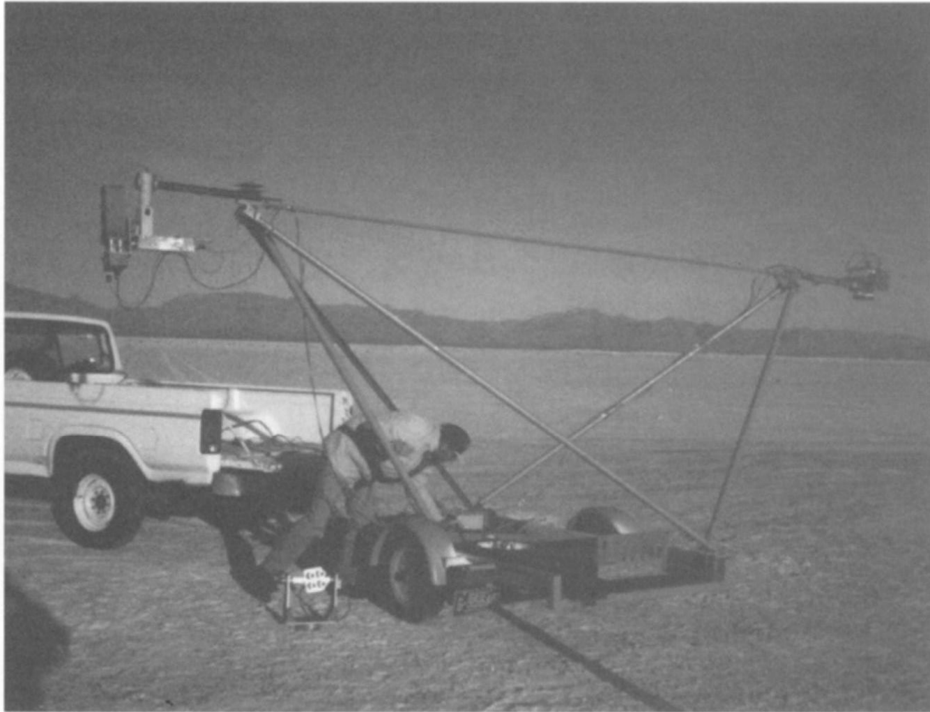
Figure 6.11 The reflectomobile used by Slater et al., 1987, in calibration of satellite sensors. The radiometers are calibrated in the field with reflectance standards and then driven over a study site to generate mean reflectance over a large, approximately uniform surface. (Courtesy of Phil Slater, University of Arizona.)
